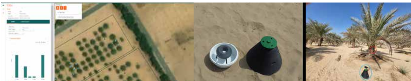
Figure 7: Example of the system tested with AgriIoT traps for RPW control and the geospatial agricultural and real-time data management platform, AgriIoT. On the left, the pheromone trap shown in the blue oval is a pheromone trap amended by the RPW counting scanner connected to a mobile app.
